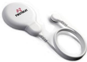
Figure 2. Firstbeat Bodyguard wearable RR intervals recorded based on ECG signal acquisition with disposable electrodes
