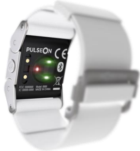
Figure 2. PulseOn sensor solution combines green and IR light with optimally matched LED-PD distances.
