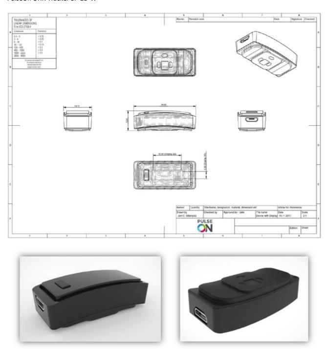
The product is designed to have three strap lengths. On the picture below are the dimensions for medium (M) size strap with total length of 245 mm (small 195 mm and large 275 mm). Dimensions can be modified based on customer needs.
