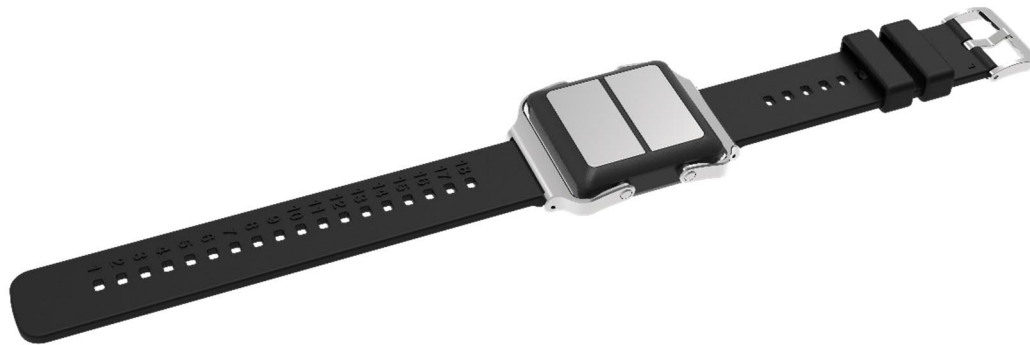
Figure 1. Wrist-worn arrhythmia monitoring device used in the study.
