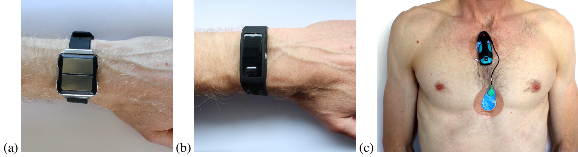
Figure 1. The wearables under test: (a) PulseOn Arrhythmia Monitor (Pulseon Arr); (b) PulseOn Optical Heart Rate Tracker (PulseOn OHR); and (c) Bittium Faros 180 chest patch (Faros 180).
